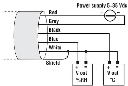
The instrument is equipped with a 7 wire + shield cable. The **Yellow** and **Green** wires are used during calibration only for PC connection through the HD9817T.1CAL interface module (see the paragraph about the RH sensor calibration).
